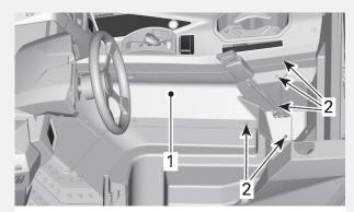
REAR PORTION OF THE LH LATERAL CONSOLE PANEL LH lateral console pane
