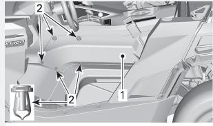
FRONT PORTION OF THE LH LATERAL CONSOLE PANEL LH lateral console pane
